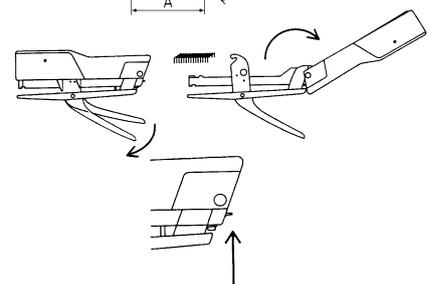
**Patented anti-jamming device.**
